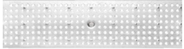
Perforated grating , galvanised, stainless steel Load classes: A15, C250, Length: 50 cm, 100 cm, Ø 6 mm
