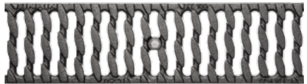
Slotted grating, Oval Grip Design , cast iron, cataphoretic dip coating Load classes: C250, E600*, Length: 50 cm, SW 10 mm
