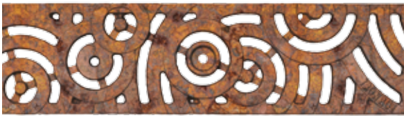
Design grating, CELTIC , cast iron Load classes: C250, Length: 50 cm, SW 10 mm
