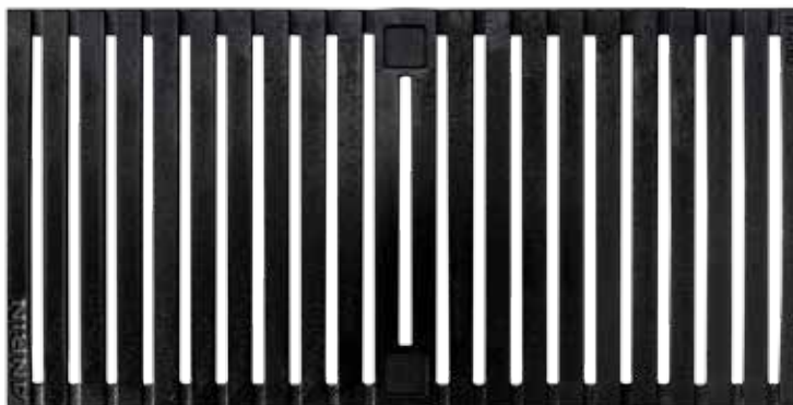
Slotted grating, HEELGUARD , cast iron, cathaphoretic dip coating, coated in black Load classes: D400*, Length: 50 cm, SW 6 mm
