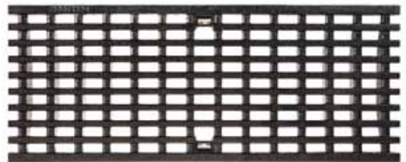
Longitudinal Grating , cast iron GJS, cataphoretic dip coating Load classes: D400*, E600*, Length: 50 cm, MW 25 x 11 mm
