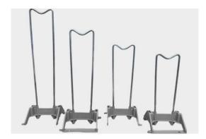
**Type B High Chairs** are used in thicker slabs. The Chair base in standard for all sizes up to 20" and is made from high impact material. The cradle is made with 1/4" wire. Lightweight for handling yet strong and stable.
